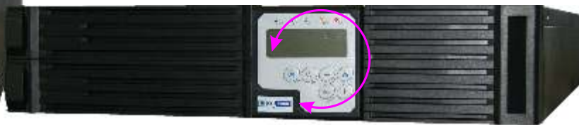
Rack to Tower Display
